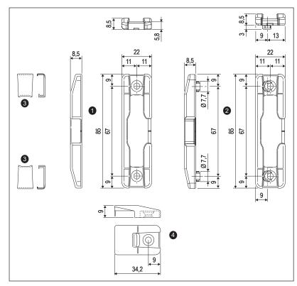
12 mm gap, 13 mm axis, 24 mm rebate base (30 mm rebate base version A52200.CR.70 only)
